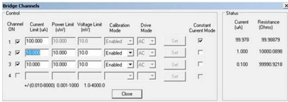
Figure 6-4. Selecting Constant Current Mode in channel 1 in the Bridge Channels Setup
